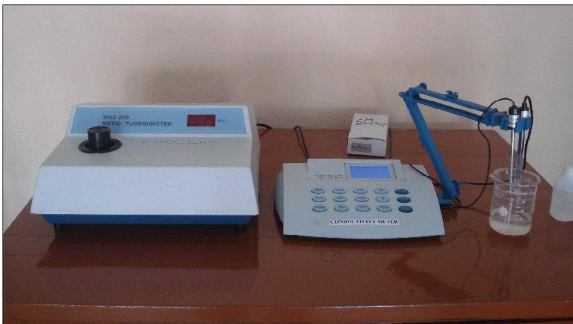
Digital Turbiditymeter detects Turbidity of water sample and Conductivitymeter measures Conductivity, Total Dissolved Solid (TDS), and Salinity of soil & water sample
