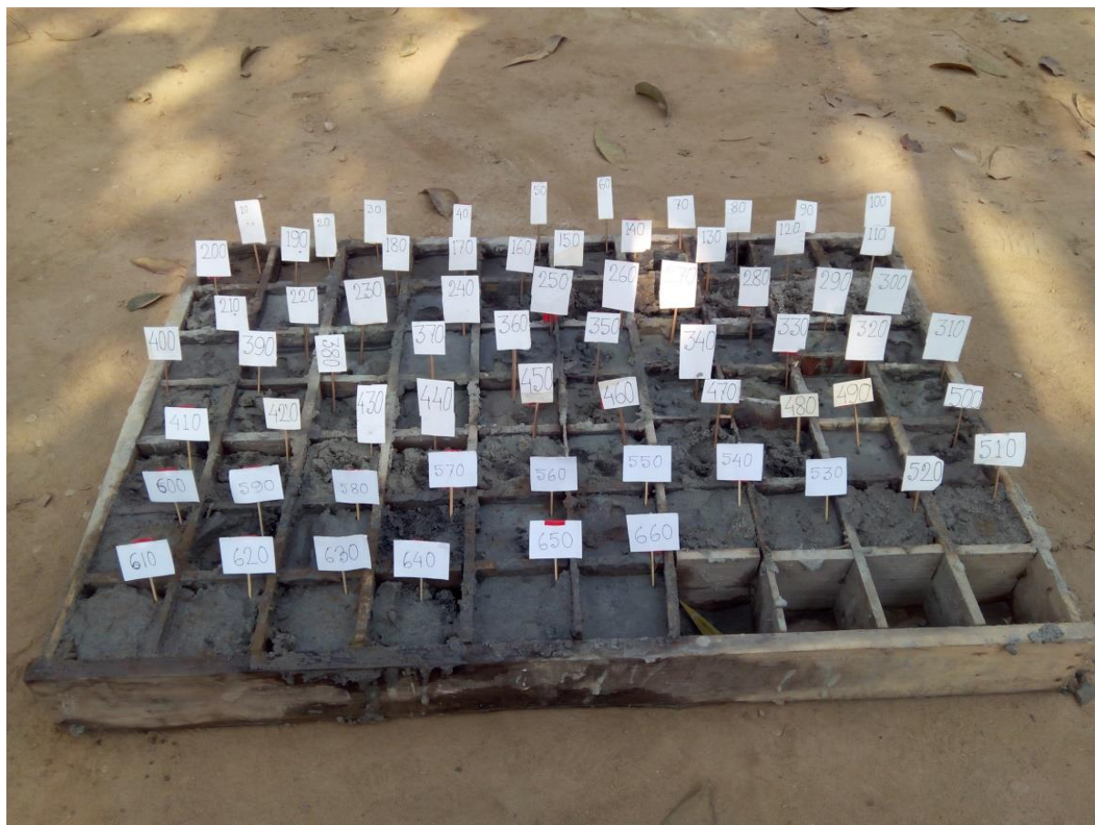
Figure 4-8: Sediment Sample Collection during Exploratory Drilling
