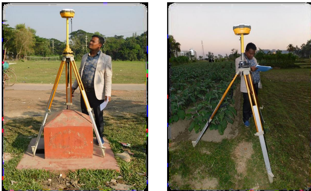
Figure 5-5: RTK Base Station, SOB Geodetic Pillar (Left) and RTK Survey at Corner of a Plot (Right)
