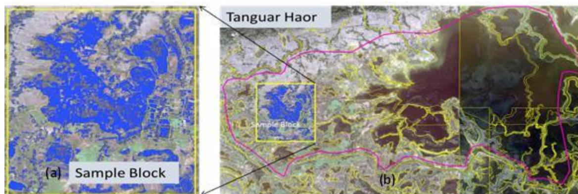
Figure 5-7: (a) The Result for Unsupervised Classification Technique (enlarged) for the Sample Block; (b) The Area of Sample Block (Shown in Rectangle Marked by Yellow Line) for Which Unsupervised Classification was Conducted
