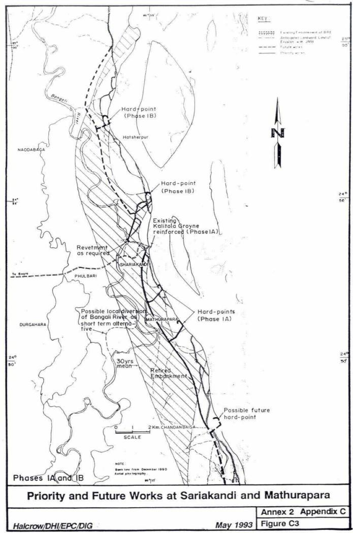
89°4d 89° 35 Possible future hard point retired embankment 4 24° ARABARI Mean BARABILA Hard-point (Phase IC) Strategically retired embankment Hard-point (Phase IC) Khudbandi Bedgari ALAMPUR NOTE: Bank line from December 1990 KEY: Aerial photography . Possible Existing Embankment of BRE future: Anticipated Landward Limit of Erosion with JMB hard-point Future works Priority works Phase IC Priority and Future Works at Kazipur Annex 2 Appendix C Figure C4 May 1993 Halcrow/DHI/EPC/DIG
