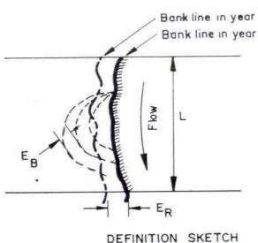
L is length of reach E<sub>R</sub> is overall bank erosion E<sub>R</sub> is bend erosion at a site t is the planning period SB is set back distance TR is trigger distance
