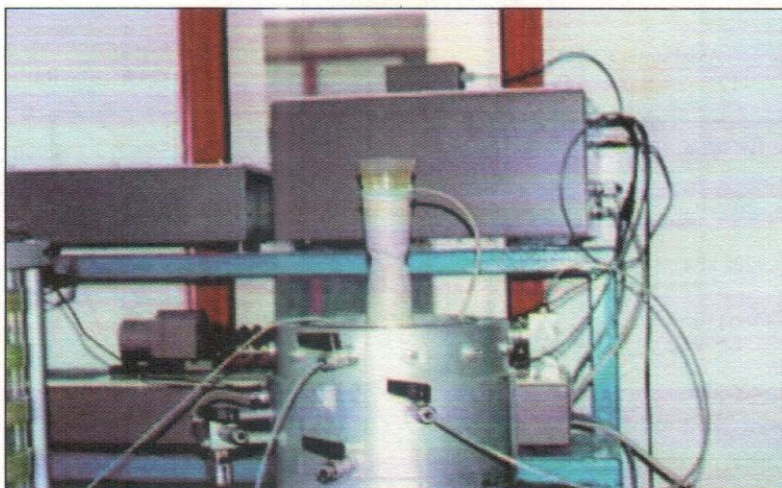
Figure 9. Photographic view of GDS triaxial testing system and failure pattern triaxial extension test specimen
