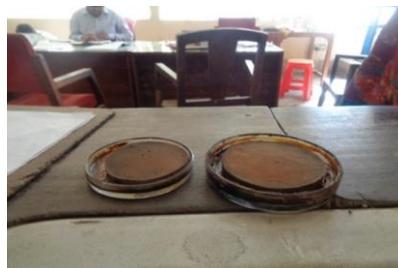
**Fig. 2.** Plasticity (Liquid limit and Shrinkage limit) measurement test
