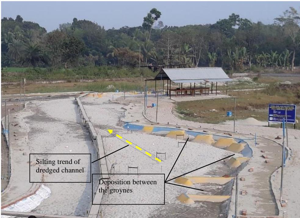
Fig. 5. Effectiveness of dredged channel, groynes & bank revetment as observed after model run (T6)
