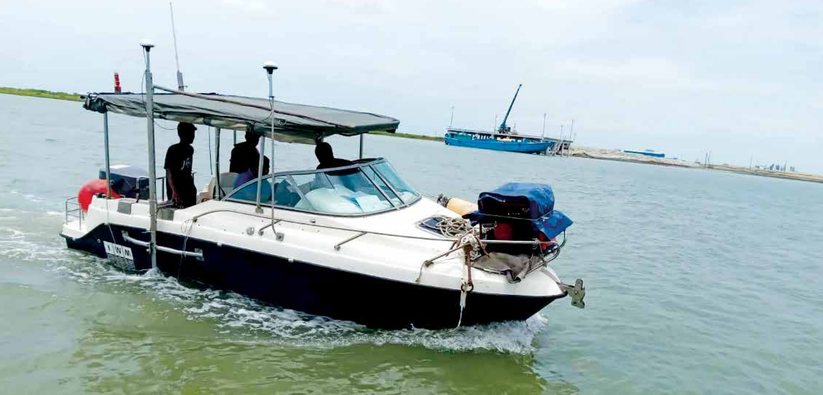
IWM survey boat carrying out multibeam survey at Kohelia River
