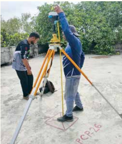
Control Point Establishment through static survey by RTK-GNSS
