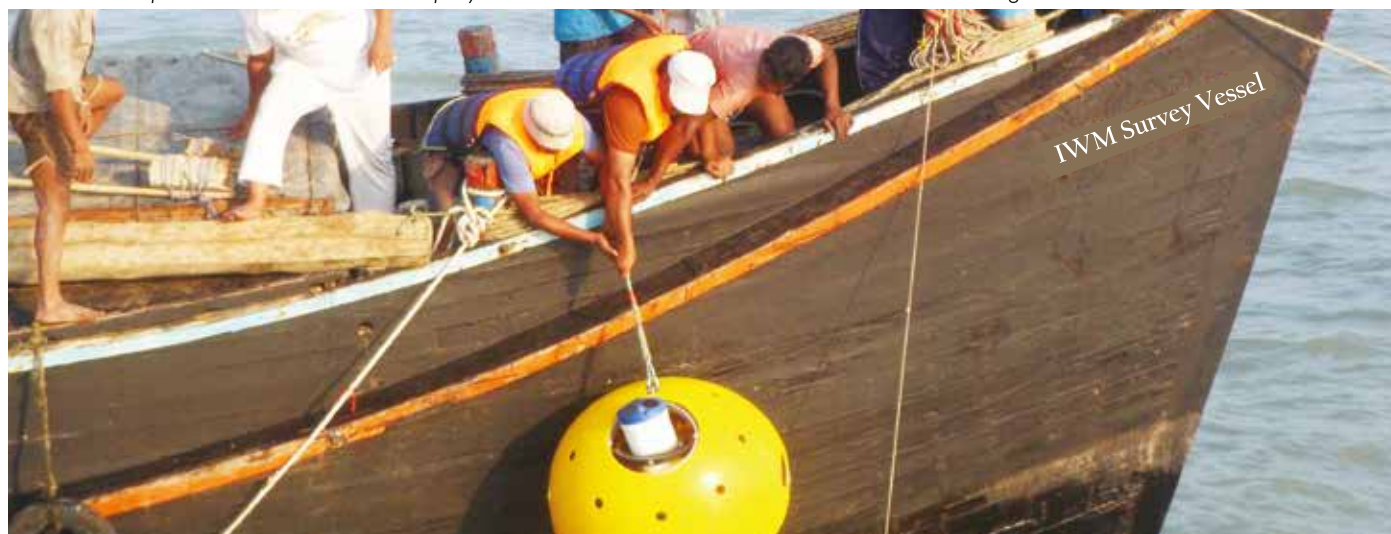
ADCP being deployed on the seabed
