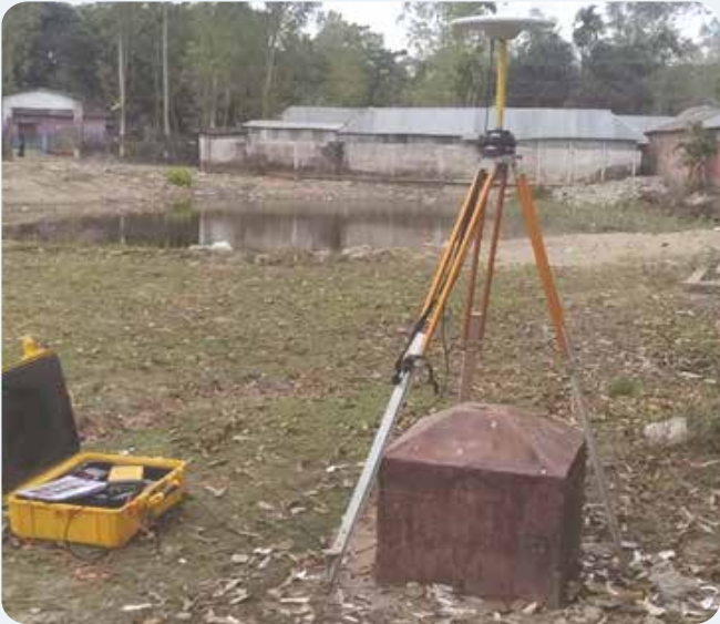
RTK-Base Station Set up on an SoB BM Pillar
