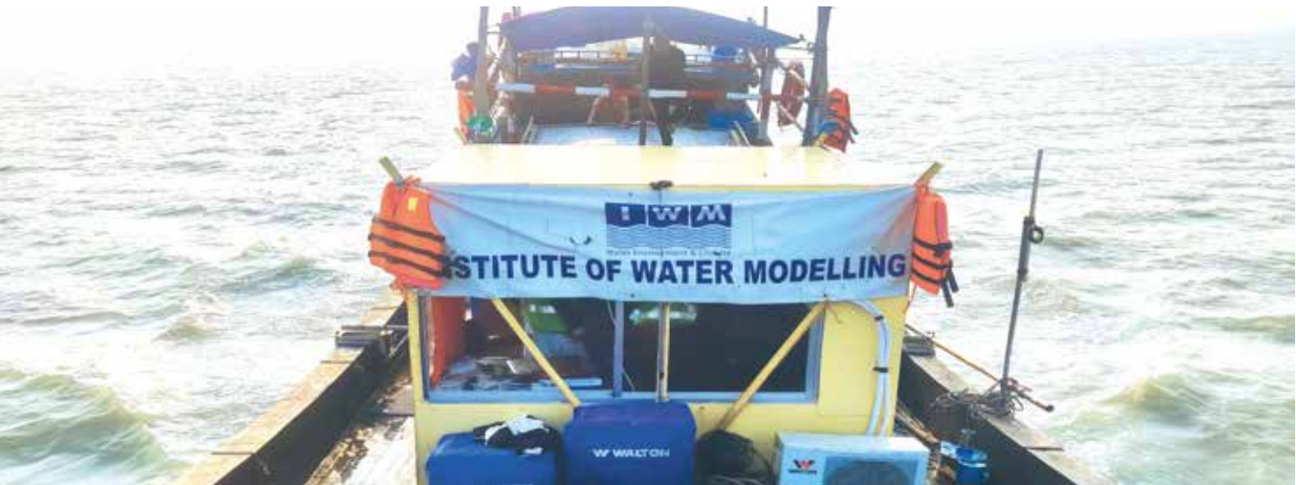
Fishing Trawler modified for Multibeam Echosounder Boat for Kutubdia Channel
