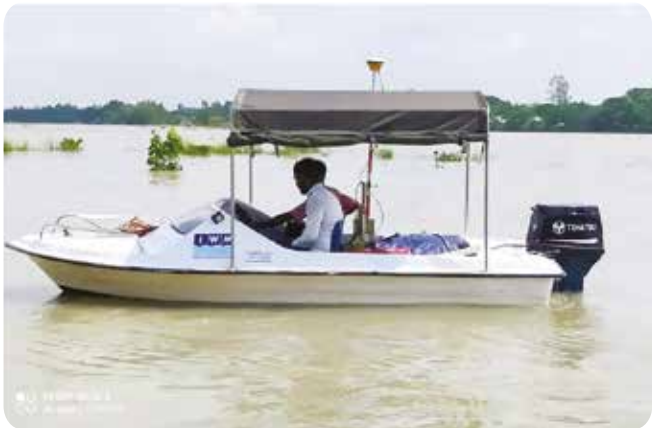
Bathymetric Survey Boat deployed in Old Brahmaputra Dredging Work (IWM Survey vessel-1)
