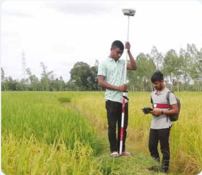
RTK-GPS Data collection at Site
