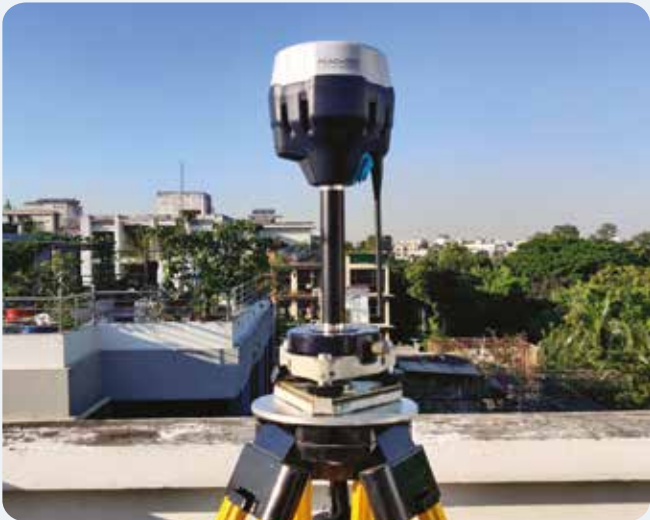
RTK-Base Station Setup on Rooftop
