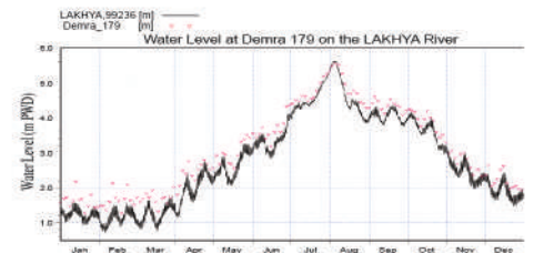
Calibration of Model at Demra on Lakhya River
