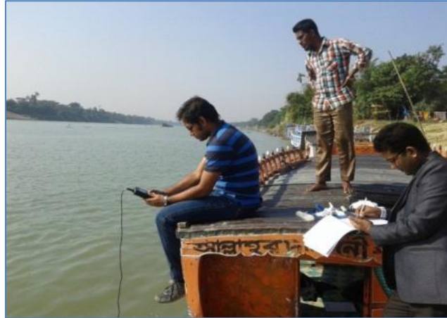
Figure 6.12: RRI personnel testing water quality parameters using HACH 30 QD Multiparameter at Sachna Bazar location of Surma River
