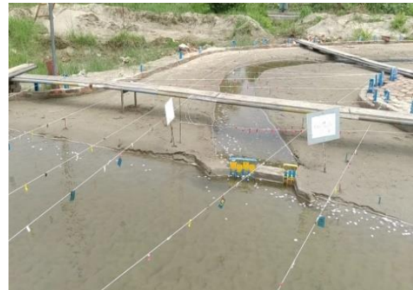
Fig. 17. Flow through the existing and proposed regulators in the model (T5).
