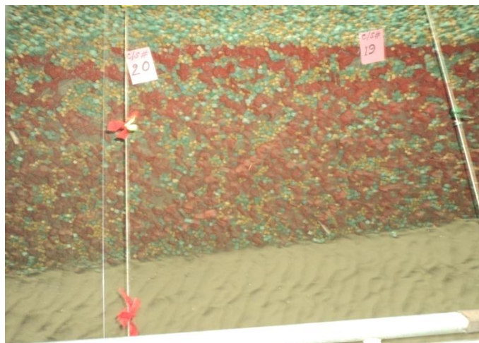
Figure 5.22.3: Launching pattern after test run (T18)
