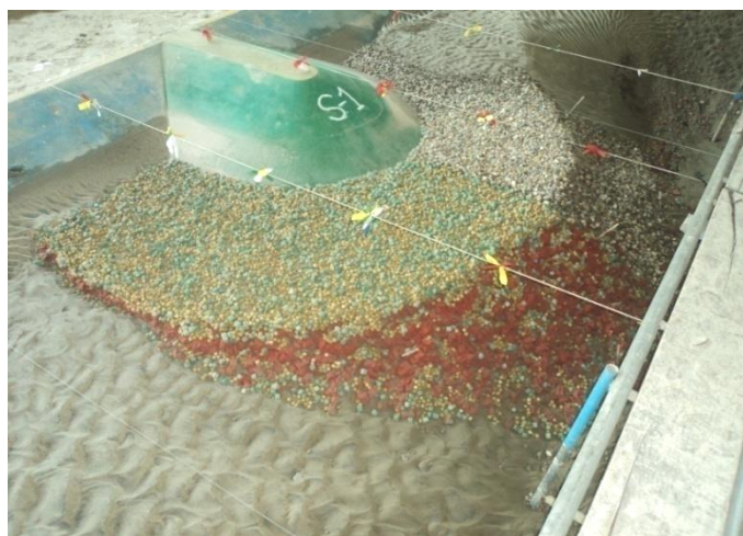
Figure 5.24.3: Launching pattern after test run (T20)
