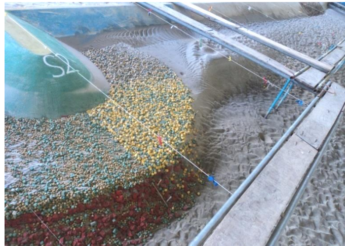
Figure 5.26.4: Launching pattern after test run (T22)
