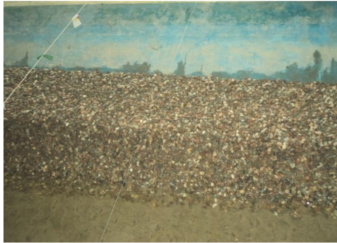
Figure 5.6.3: Launching pattern after test run (T4.2)
