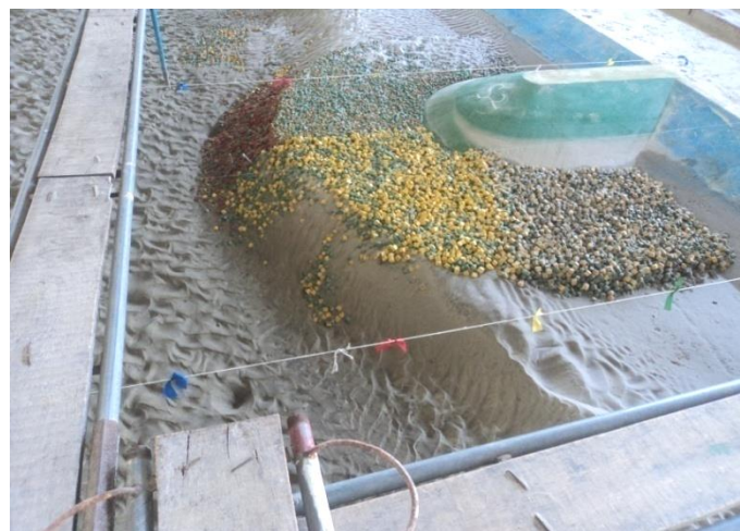
Figure 5.25.4: Launching pattern after test run (T21)
