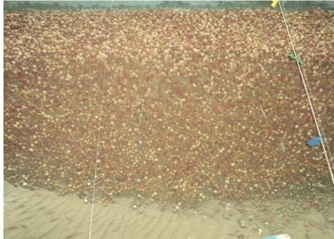
Figure 5.11.3: Launching pattern after test run (T7)
