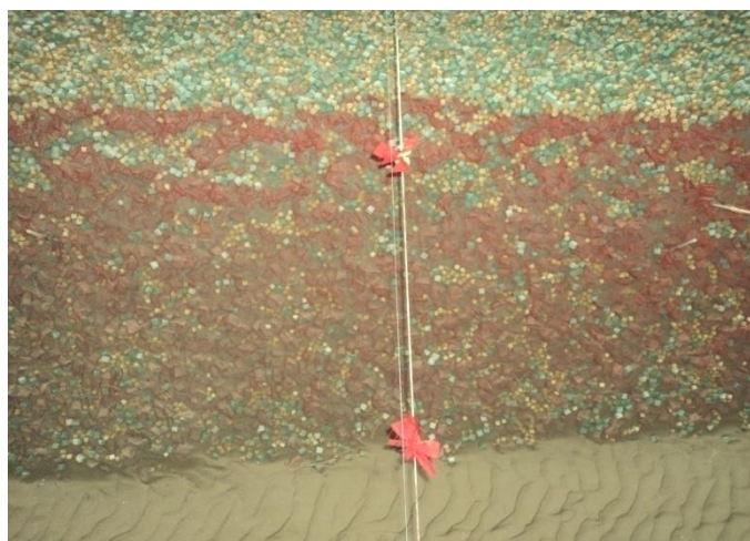
Figure 5.21.3: Launching pattern after test run (T17)
