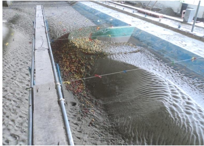
Figure 5.26.3: Launching pattern after test run (T22)
