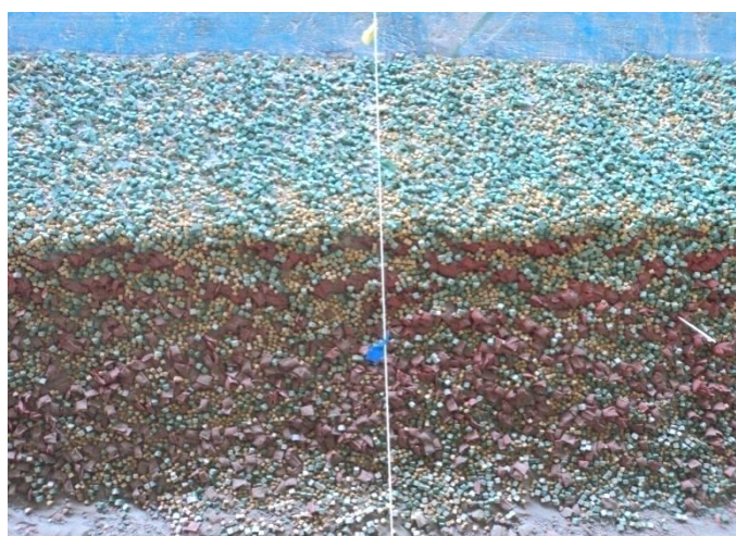
Figure 5.16.3: Launching pattern after test run (T12)
