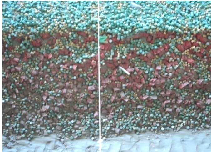
Figure 5.18.3: Launching pattern after test run (T14)
