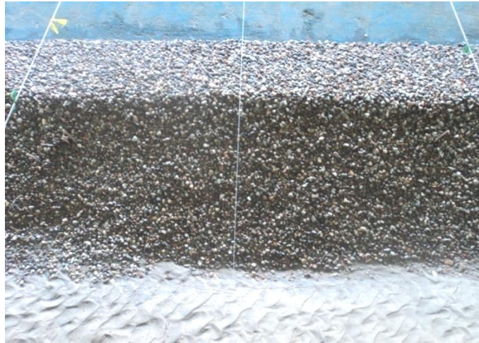
Figure 5.12.3: Launching pattern after test run (T8)
