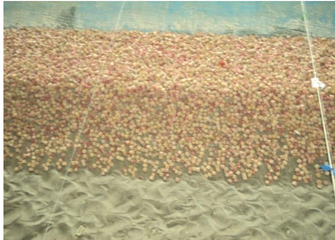
Figure 5.10.3: Launching pattern after test run (T6.2)
