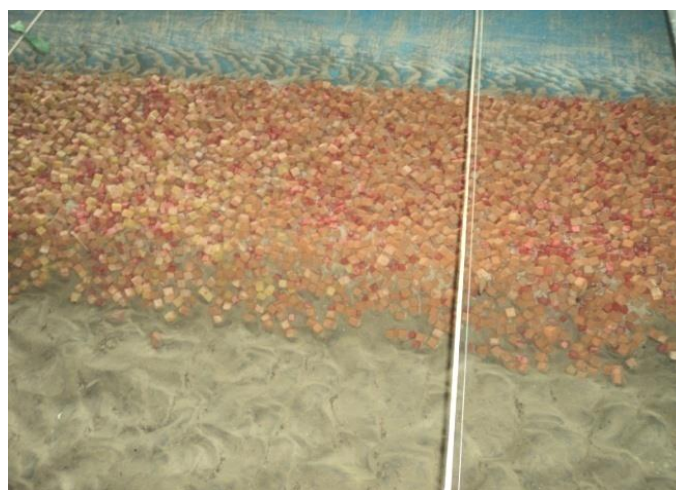
Figure 5.3.3: Launching pattern after test run (T2)
