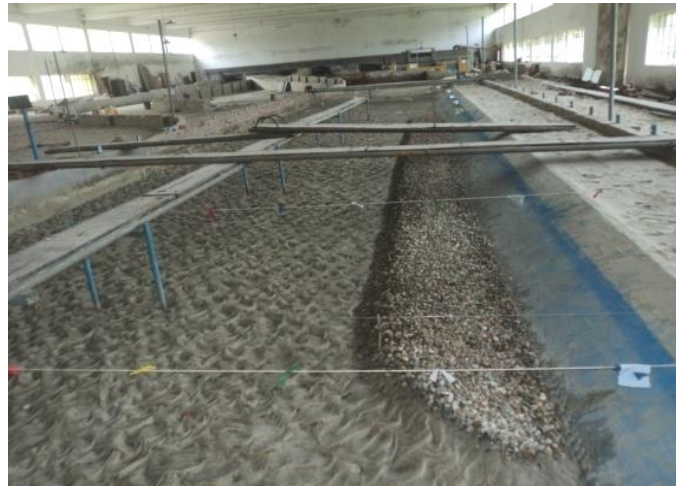
Figure 5.4.3: Launching pattern after test run (T3)
