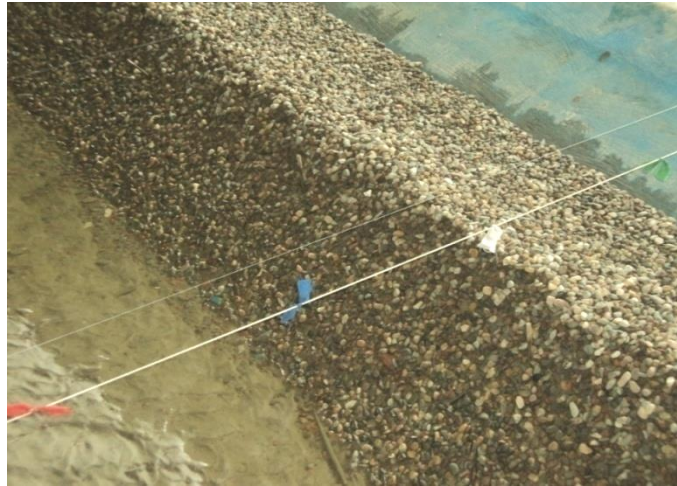
Figure 5.5.3: Launching pattern after test run (T4.1)
