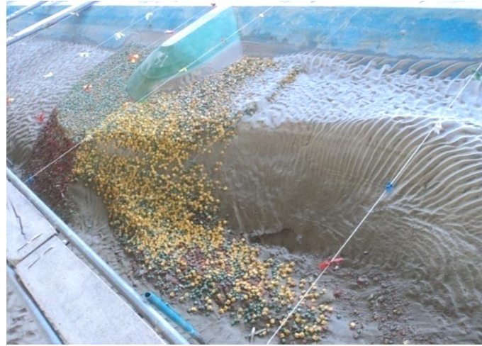
Figure 5.25.3: Launching pattern after test run (T21)
