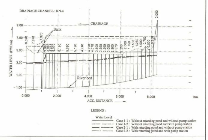
FIG. D.14 PROFILE OF SIMULATED PEAK WATER LEVEL OF NARAYANGANJ DND
