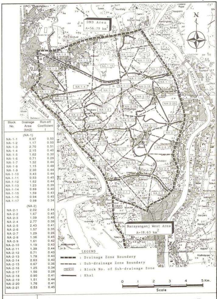
SUB-DRAINAGE ZONE AND THEIR RUN-OFF COEFFICIENT : DND
