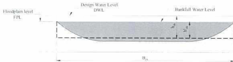
Fig. 4.4-1: Sketch of a cross-section in a straight river section
