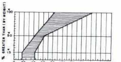
GRADING RANGE D D 50 = 25 mm (W 50 = 40 kg) Layer thickness = 50 cm
