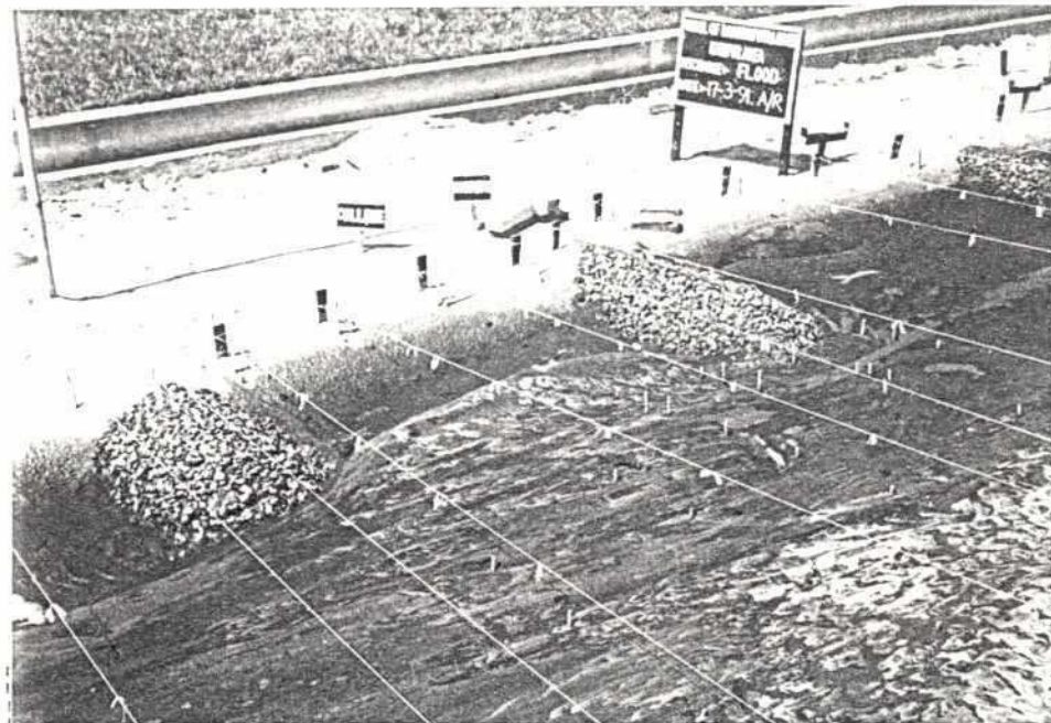
Photo 5. Test 9: Bed condition after running 100-years flood discharge (close view) showing the point of maximum scour at nose of Groyne E off the Hospital
