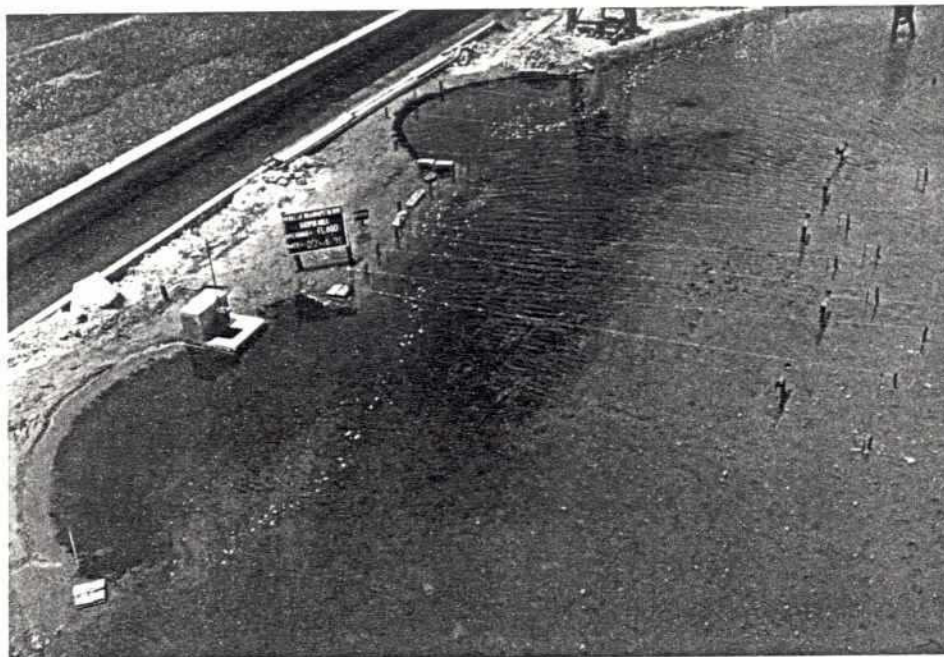
Photo 9. Test 18: Flow conditions with artificial embayment Shape-2, 100-years flood discharge
