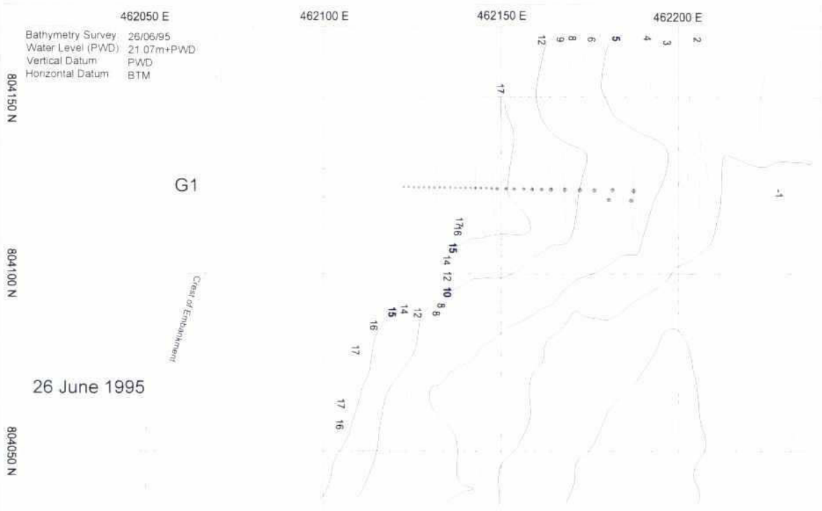
Fig. 6.8-3: Bathymetry around groyne G-1 on June 26, 1995
