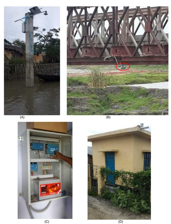
Figure 2:2: Typical equipment for Component B, (A): Water level sensor at Mongla river, (B): Water level sensor at Satkhira; (C) Real time data transfer equipment (D) Protection room housing equipment, Satkhira
