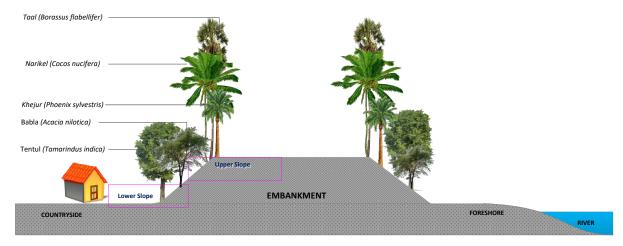
Figure 4.2: Typical Cross Section of embankment slope afforestation works
