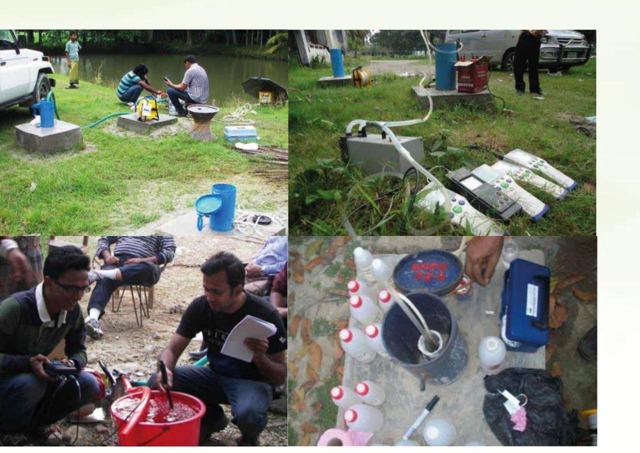
Figure 10: Measurement of physical parameters of groundwater in the field and collection of water samples for laboratory analysis.
