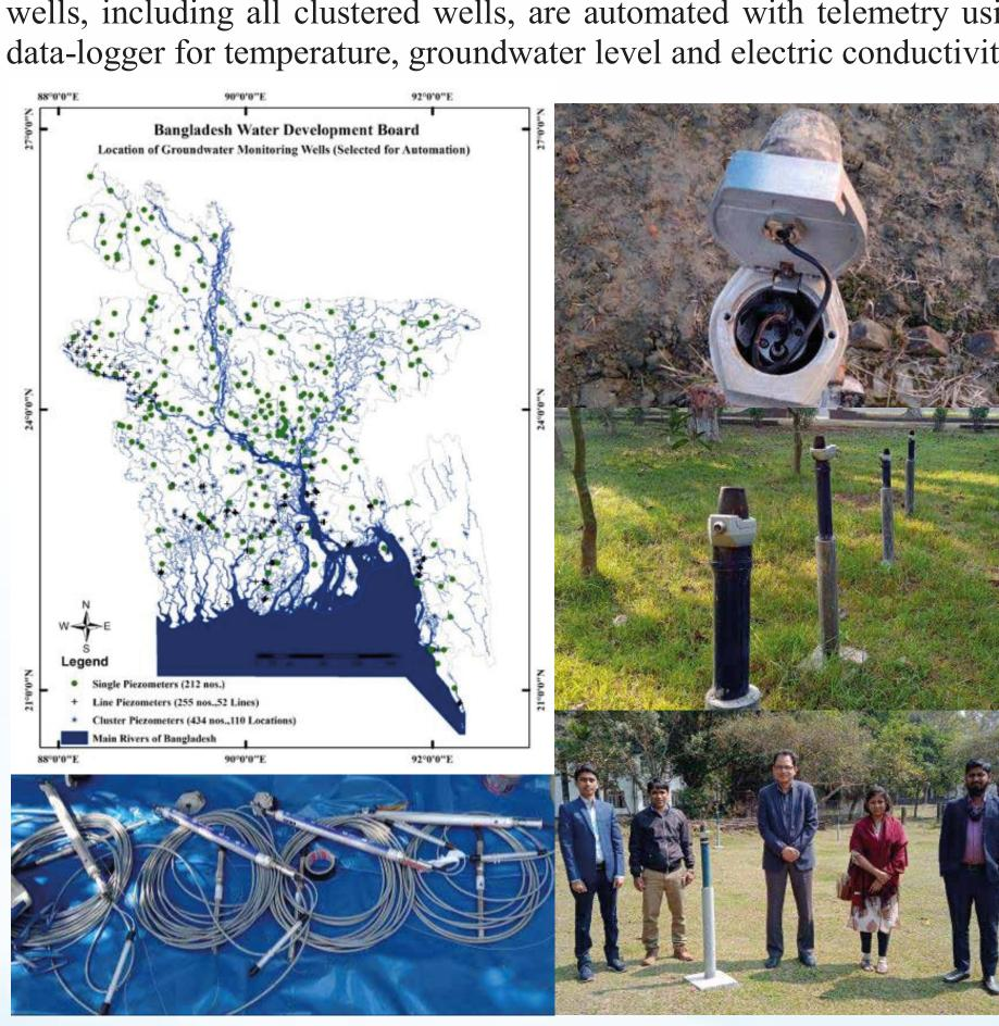
Figure 8: Locations of 905 nos. automated groundwater monitoring wells with telemetry for real time data transmission throughout Bangladesh.
