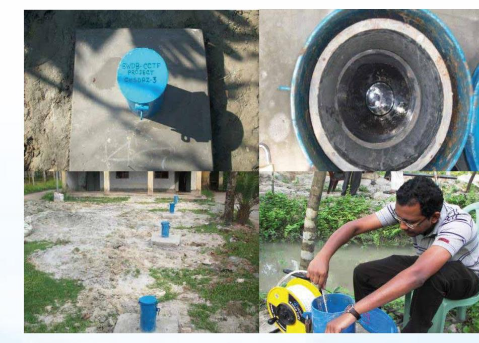
Figure 6: Examples of clustered groundwater monitoring wells in the coastal areas of Bangladesh.
