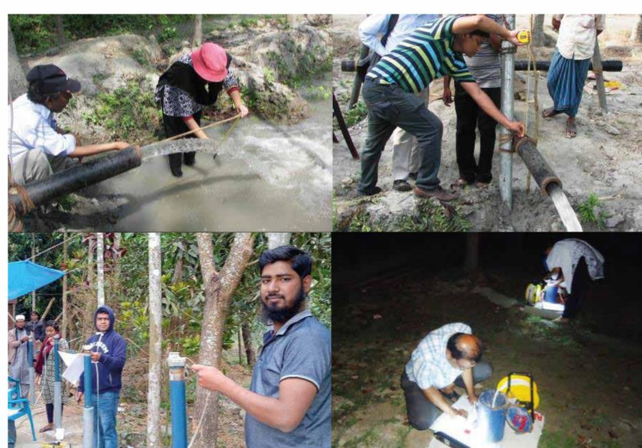
Figure 9: Performance of aquifer pumping tests to determine hydraulic properties of aquifer sediments.
