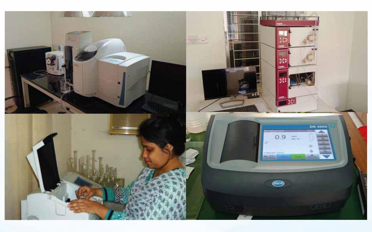
Figure 12: BWDB laboratory equipped with Atomic Absorption Spectrophotometer, Ion Chromatograph, UV-VIS Spectrophotometer, Spectrophotometer and other instruments for water quality monitoring.
