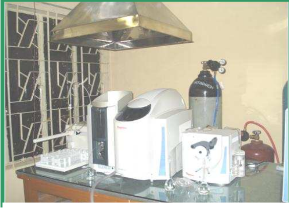
Atomic Absorption Spectrophotometer in the Chemical and Water Pollution Lab under Geotechnical Research Division for determining heavy metals
