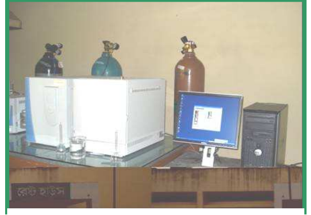
Gas Chromatography Mass in the Chemical and Water Pollution Lab under Geotechnical Research Division for determining the organic compounds
