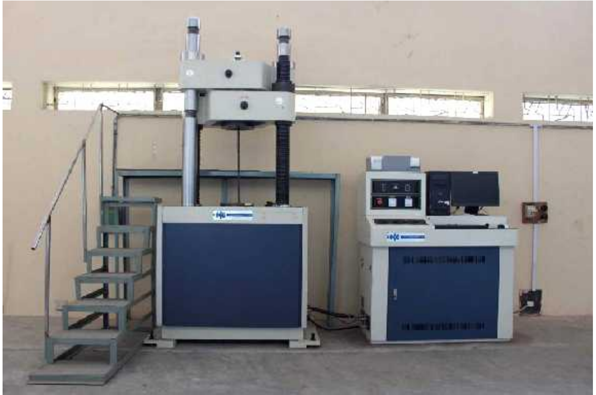
The Universal Testing Machine (UTM) for testing of MS rod, flat bar, concrete cylinder, block etc
