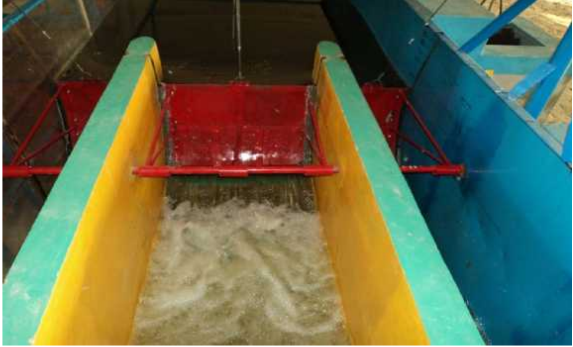
Nature of flow in the stilling basin with jump over the glacis for unit discharge
