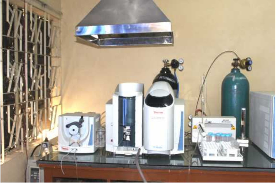
Atomic Absorption Spectrometer for determining metals such as Al, Ba, B, Cd, Cr, Mg, Fe, As, Hg etc.
