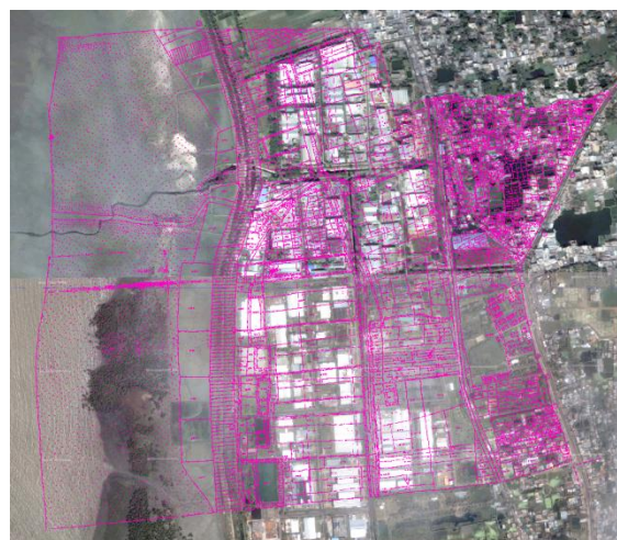
Figure 3-11: Geo-rectification of Mouza sheet using Satellite Images
