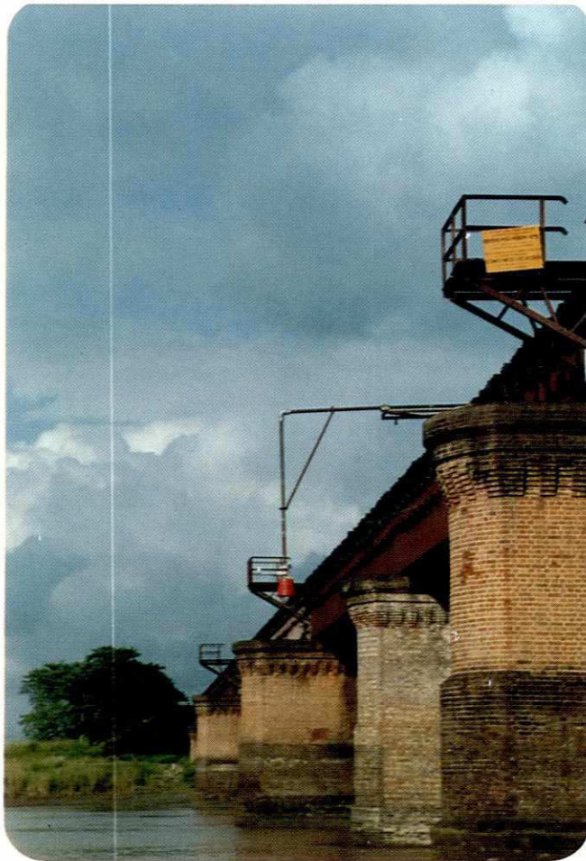
b. Mounted acoustic type AWLR on one of the piers of Mymensingh Railway Bridge
