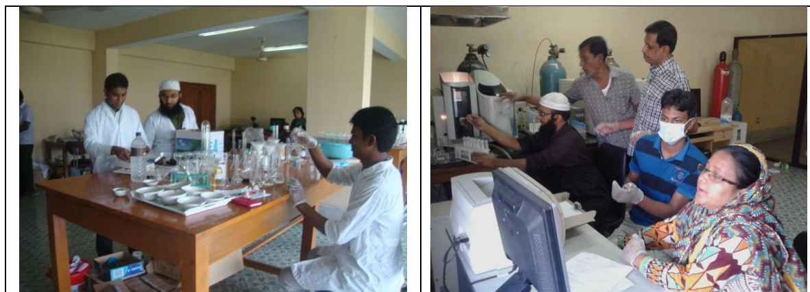
Figure 3.14: Sample preparing for metals analysis (left) and detecting metals using AAS at the lab (right).
