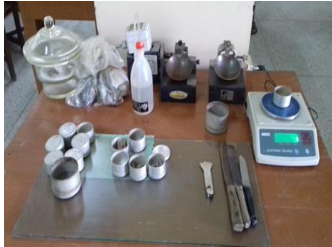
Figure 3.27: Arrangement for Atterberg Limits test
