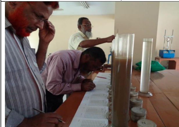
Conducting Hydrometer test at laboratory
