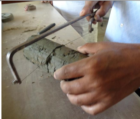
Sectioning of Undisturbed Soil samples for different tests
