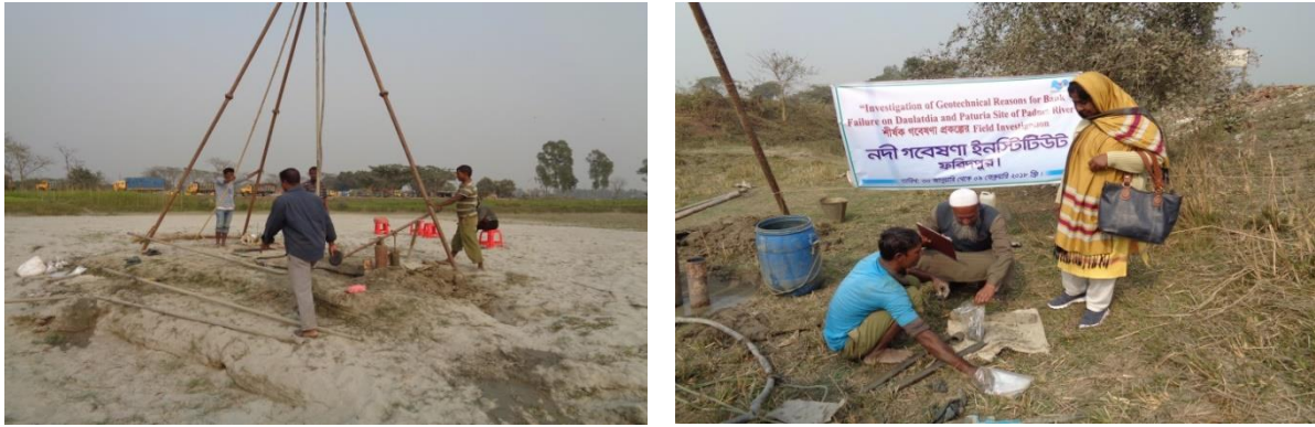
Figure 3.17: Wash Boring setup and disturbed soil sample collection using split spoon sampler
