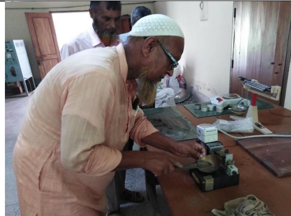
Conducting Liquid Limit test
