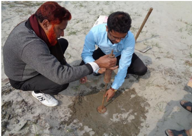
Conducting Field density measurement
