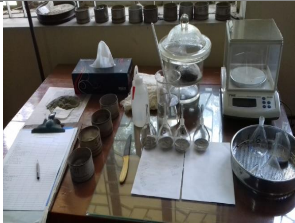
Apparatus arrangement for Specific Gravity test
