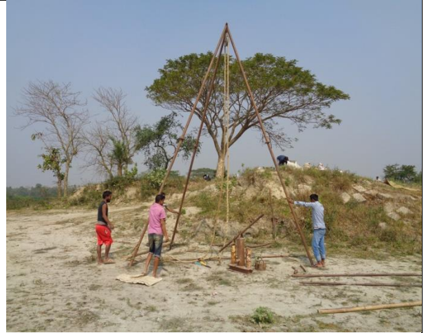
Arrangement for sample collection by wash boring method
