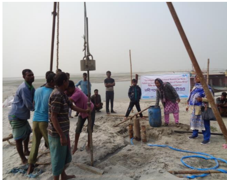
Figure 3.21: SPT count for each 6 inch penetration of soil
