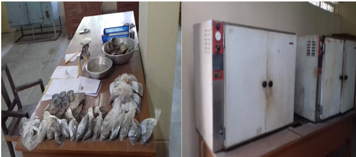
Figure 3.26: Arrangement for determining natural moisture content
