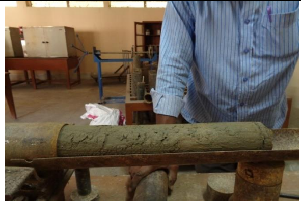
Undisturbed soil samples removed from Shelby-tube.
