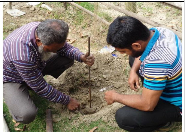
Conducting field density test in field
