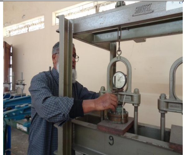
Setting soil specimen for consolidation test
