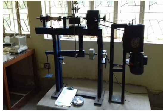
Figure 3.34: Arrangement for conducting UCT and Direct shear Test
