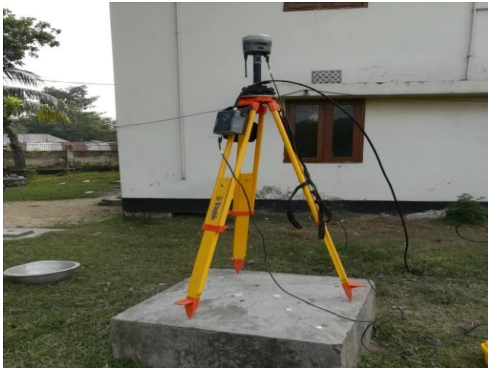
Figure 3.19: Measurement of ground level by RTK method
