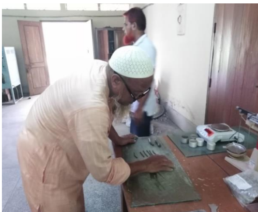
Figure 3.29: Plastic limit and Liquid limit tests at laboratory
