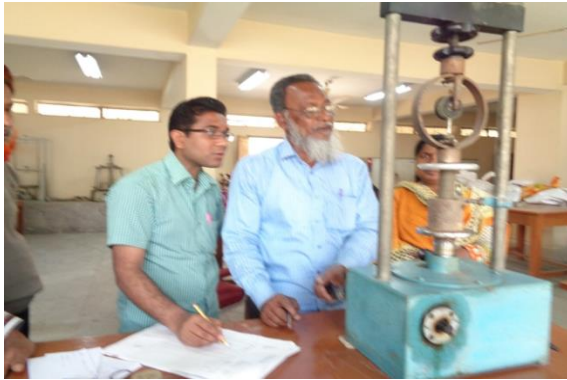
Figure 3.34: Arrangement for conducting UCT and Direct shear Test
