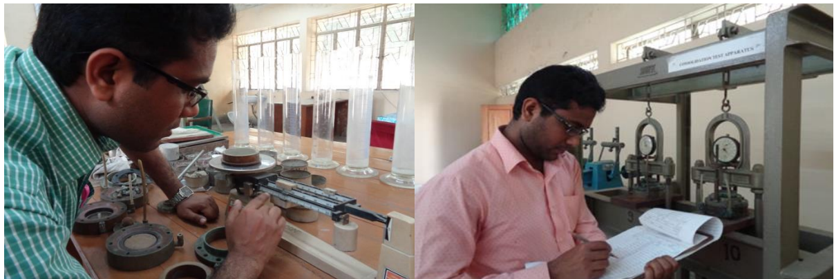
Figure 3.37: Consolidation test for settlement analysis
