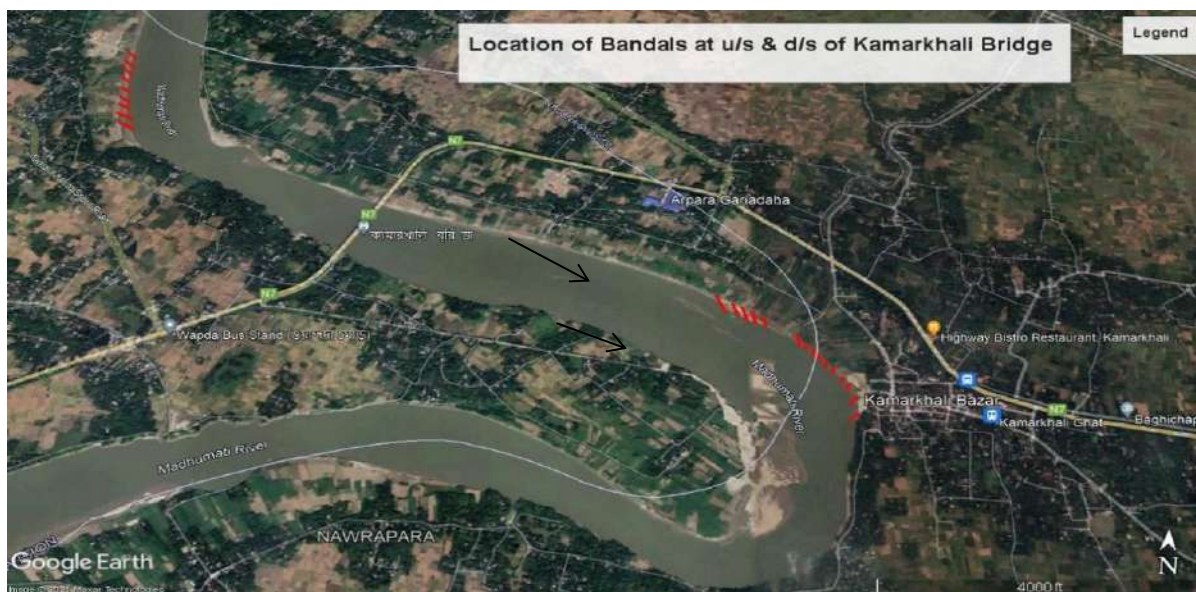
Figure 4.6 Location of the bandal structures at u/s & d/s of Kamarkhali Bridge
