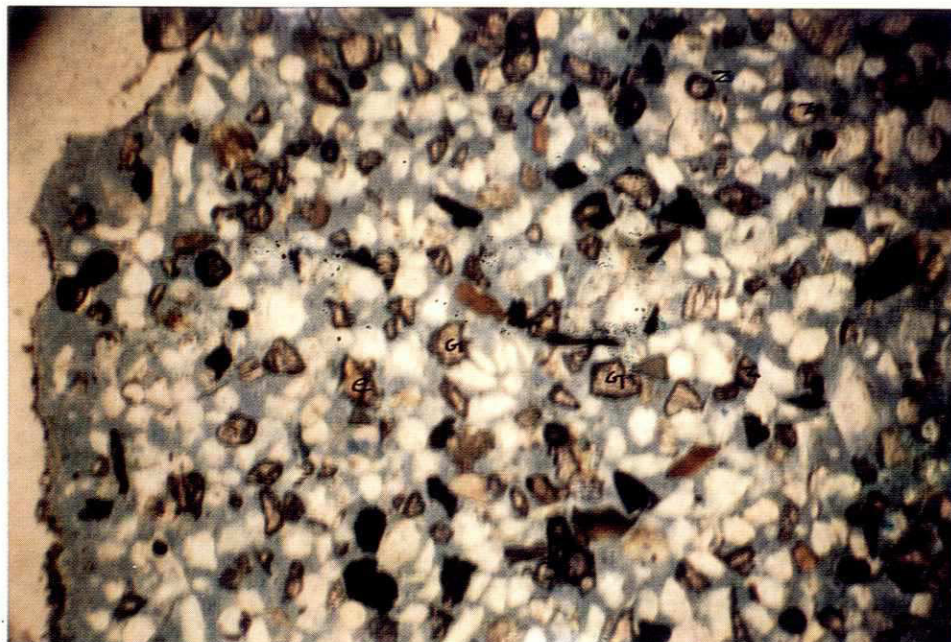
Plate 10 : Heavy minerals in Teesta confluence after flood season G = Garnet , E = Epidot , Z = Zircon (vertical height of photograph : 2.0 mm)
