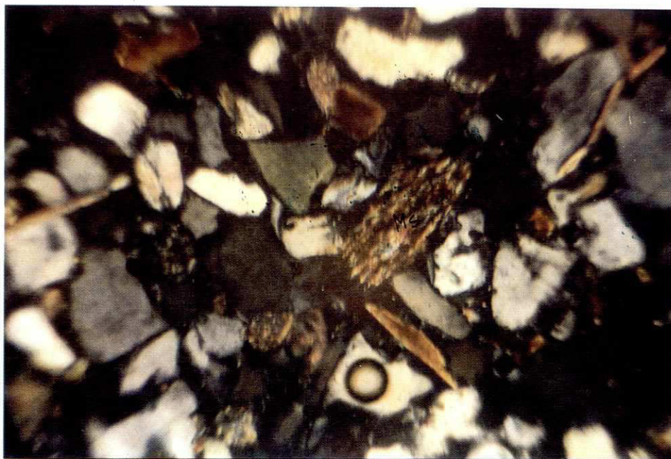
Plate 7 : Jamuna (Sirajganj) MS = mica schist lithic grain (vertical height of photograph : 0.8 mm)
