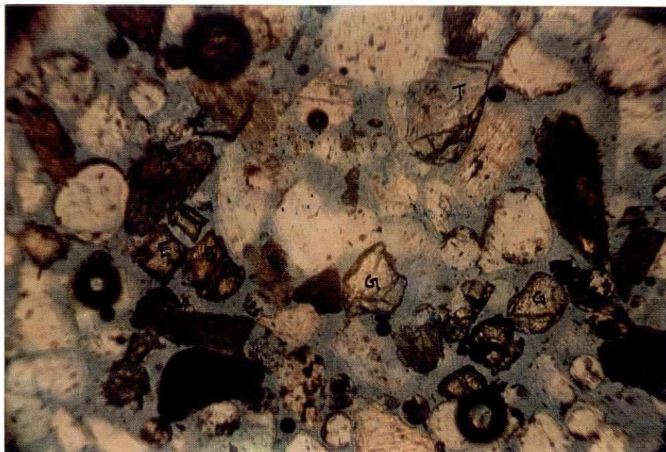
Plate 14 : Jamuna (Bahadurabad) heavy minerals: G = garnet, E = epidote, T = tourmaline, Z = zircon, H = hornblende (vertical height of photograph : 0.8 mm)
