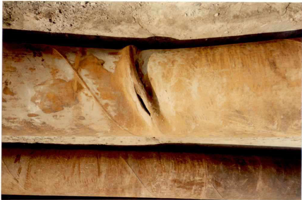
Photo 23: Groyne G-2; Tubular steel pile dia. 711.2x14.2 mm; material failure at max. deformation point about 6 m from pile tip
