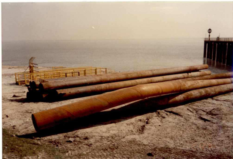
Photo 22: Groyne G-2; Tubular steel piles dia. 711.2x14.2 mm recovered from damaged part of groyne
