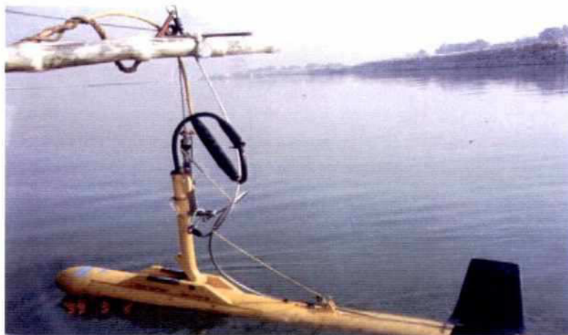
Fig. 3.4-1: Side scan sonar towfish
