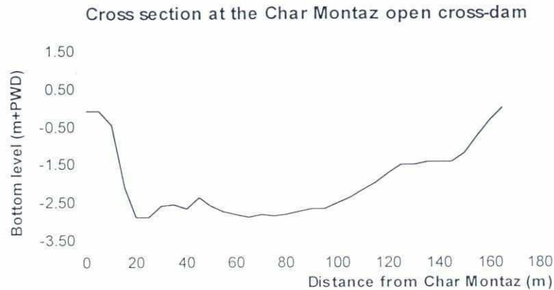
Fig-A4. Cross section at the Char Montaz open cross dam location
