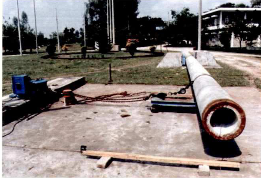
Photo 4.1-2: Pre-stressed Spun Concrete Pile; Bending Test
