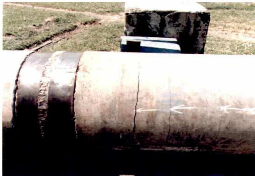
Photo 4.1-3: Pre-stressed Spun Concrete Pile; Bending Test
