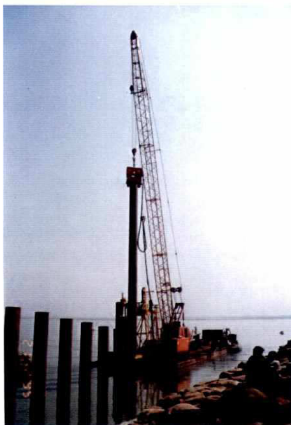
Photo 3.2-2: Floating equipment: - Manitowoc crawler crane (150 ton capacity) - Float Barge (BG7) 400 ton capacity
