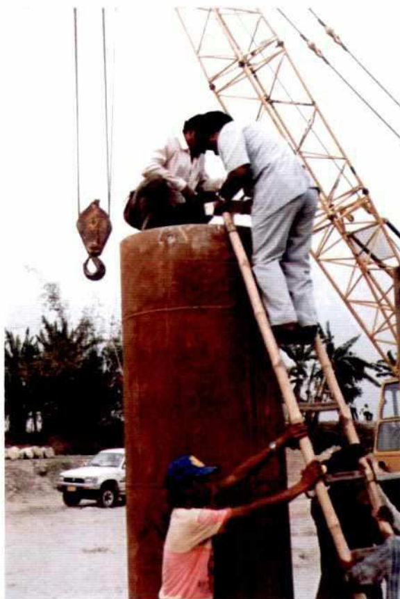
Photo 7.14-5: Pile Integrity testing of In-Situ Bored Piles
