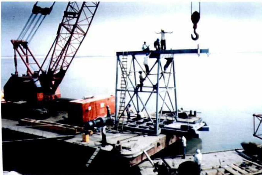
Photo 3.2-1: Floating equipment: - Manitowoc crawler crane (150 ton capacity) - Float Barge (BG7) 400 ton capacity
