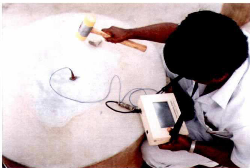
Photo 7.14-6: Pile Integrity testing of In-Situ Bored Piles; Measurement of the Stream Wave generated by Hammer Impact
