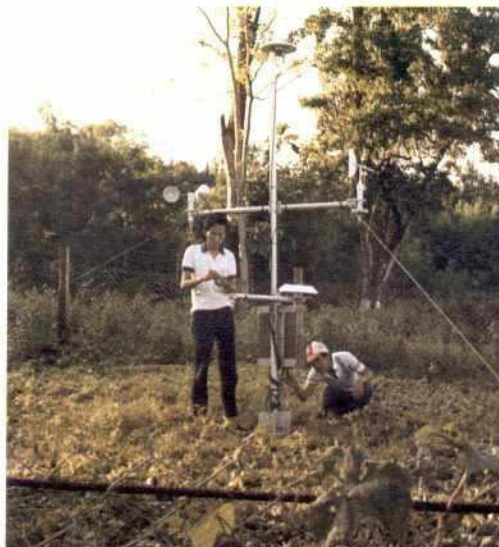
Automatic climate station: measures solar radiation, net all-wave radiation, wind speed and direction, temperature, humidity and rainfall intensity.
