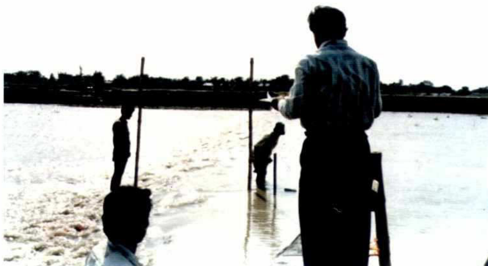
Photo 4.2-9: Flow measurements at the overtopped earth dam in June 1997
