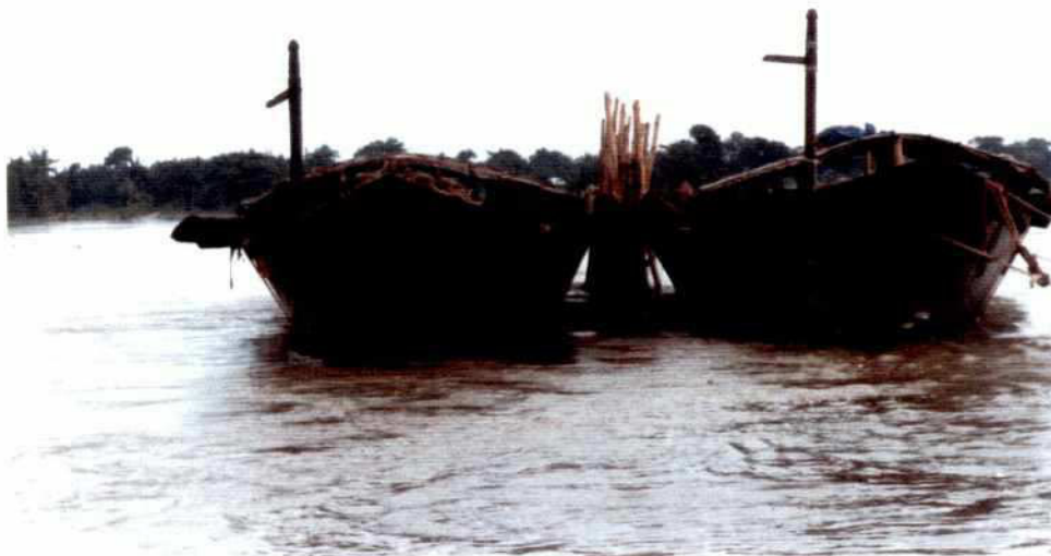
Photo 4.2-5: Floating screen test in the Fulchari channel with country boats near the bandal site at Katlamari, July 1997
