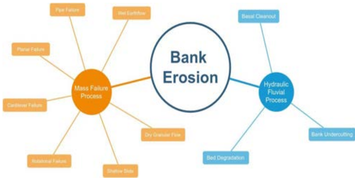
Figure 2.3 Processes of Bank Erosion
