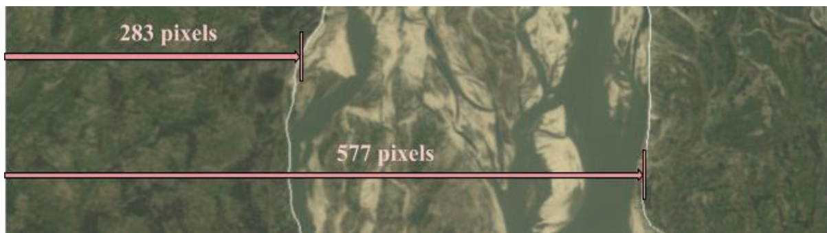
Figure 6.7 Coordinate System for defining Bank Line Locations
