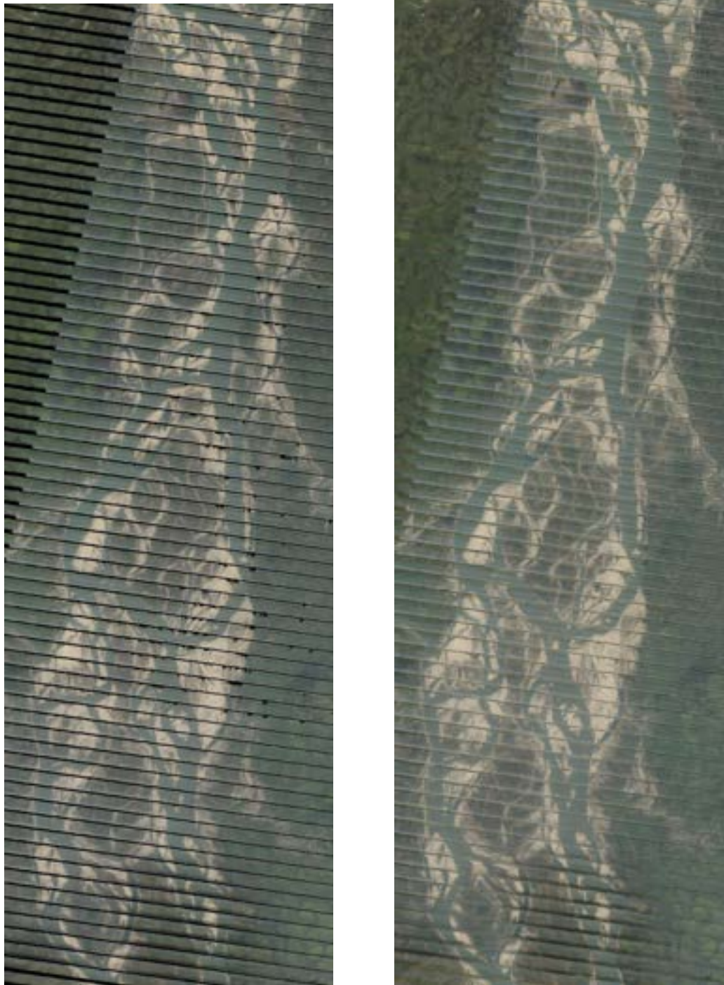
Figure 6.3 SLC off image data gaps replaced by mean values (Before and After)
