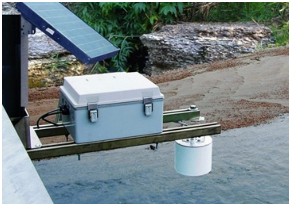
Fig 5. Representative picture of pole mounted Automatic Water Level Gauge with long arm cantilever boom ( Type I)
