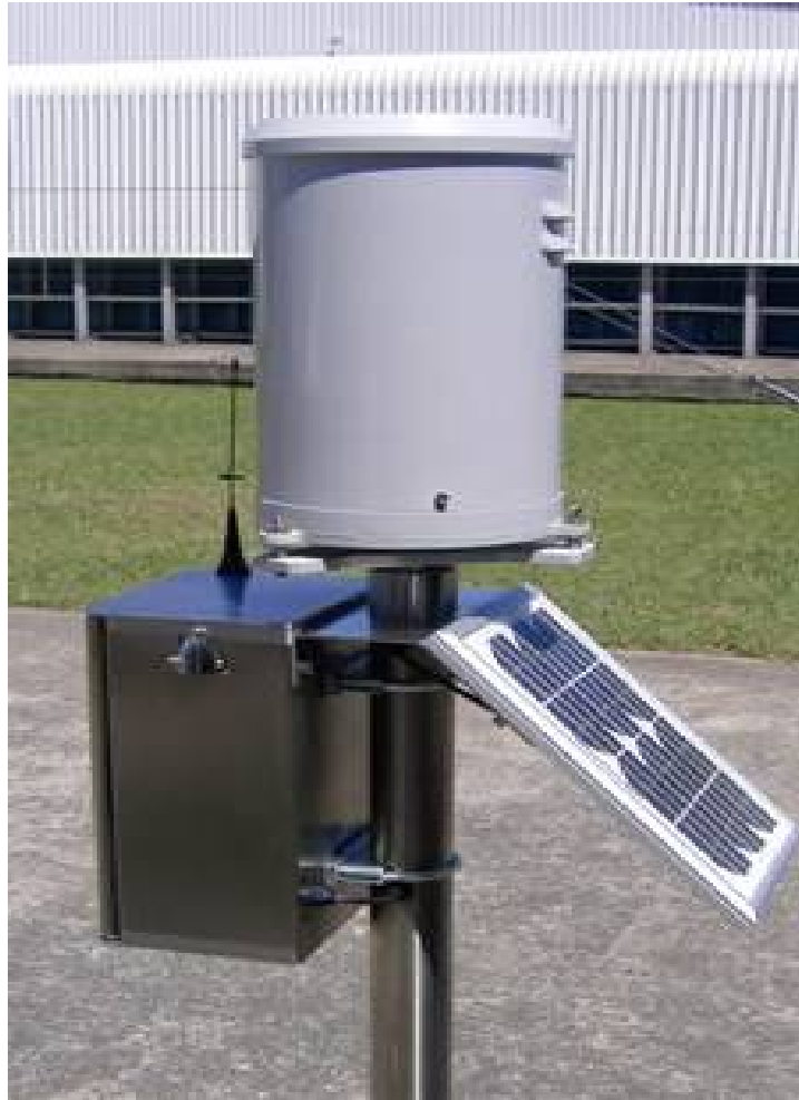
Fig 9. Sample picture of Automatic Rain Gauge (ARG) to be fixed on top of the roof
