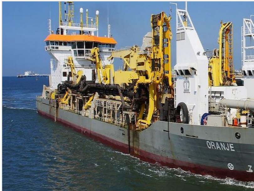
Figure 4.13: Trailing Suction Hopper Dredger
