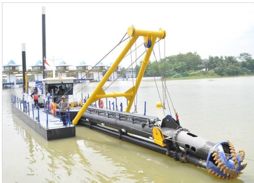
Figure 4.12: Cutter Suction Dredger
