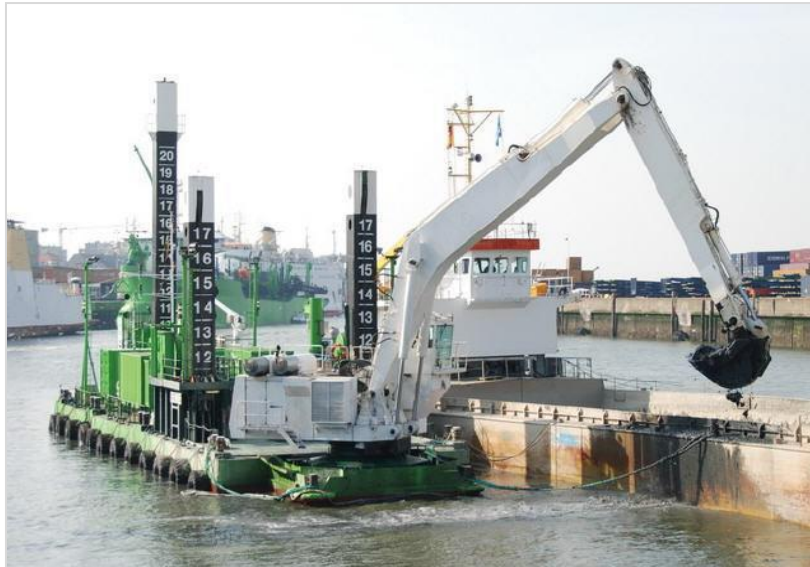
Figure 4.11: Backhoe Dredger and Barge
