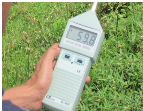
Photo 5.2: CEGIS Professional measuring Noise level during field investigation
